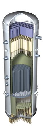
The ESBWR (Economic Simplified Boiling Water Reactor) builds on a long line of proven GEH BWR reactors. ESBWR employs passive safety design features. It is a simplified reactor design, allowing faster construction and lower operating costs.
